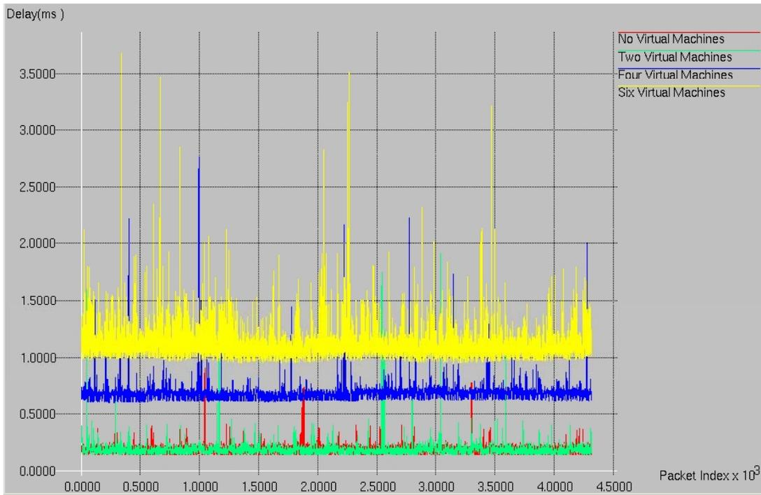
Figure 7: Measured round-trip time for ICMP echo packets
