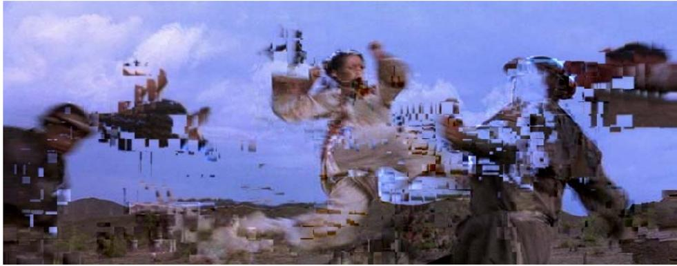
Figure 5: Mpeg4, Drop = 0.1%, Delay = 1.5 ms and Jitter = 0.025 ms
